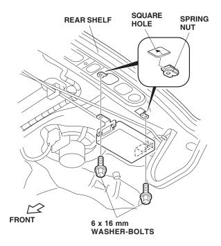
15. Mount the bass unit to the rear shelf with two 6 x 16 mm washer-bolts.
