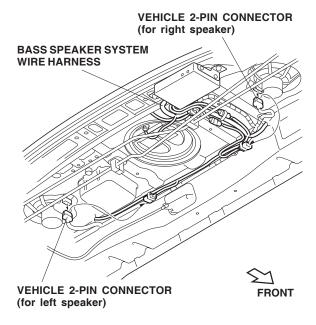
26. Plug the bass speaker system wire harness 2-pin connectors into the right and left bass speakers.
