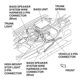
21. Plug the bass speaker system wire harness 2-pin connector (blue) into the trunk light, then connect the vehicle 2-pin connector into the bass speaker system wire harness 2-pin connector (blue) taped to the harness.
