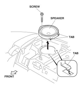
8. Install the right and left speakers using the screws removed in step 7.
