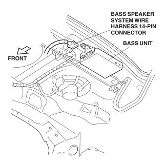
17. Plug the bass speaker system wire harness 14-pin connector into the bass unit.
