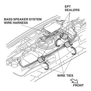
28. Using seven wire ties, secure the bass speaker system wire harness to the vehicle harness in the areas shown. Make sure that the bass speaker system wire harness does not interfere with the trunk springs during the closing and opening of the trunk lid.
